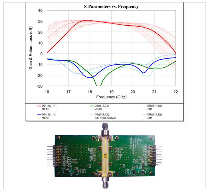
Figure 2: Simulated data including yield analysis vs. modeled small-signal frequency response for the LE-Ka1330308 reference board.
