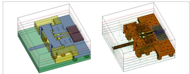
Figure 4: Details of package model I/O port simulation setup (left) and resulting mesh in Analyst software (right).
