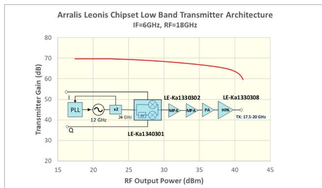
Figure 1: Chipset architecture for K/Ka-band satcom applications.
