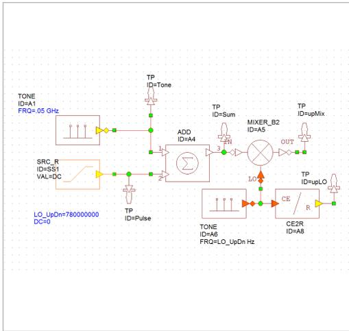
AM upconverting modulator system diagram as per course material.
