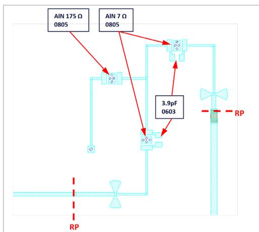
Figure 2: Equalizer network used on IMN to achieve gain flatness across required bandwidth.
