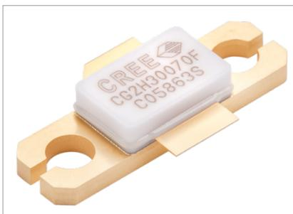
Figure 1: Compact PA solution using next-generation 28 V GaN process technology.
