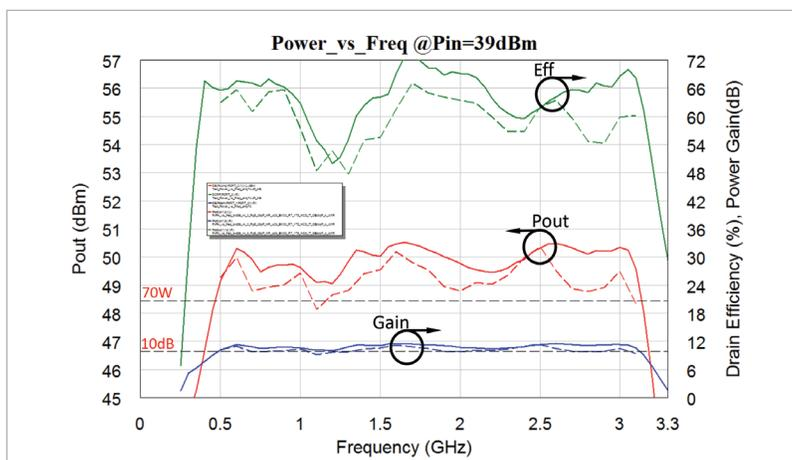
Figure 3: Measured (dashed) versus simulated (solid) data showing a high degree of correlation.
