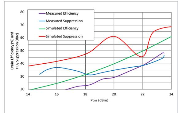
Figure 3: Optimum amplifier performance.
