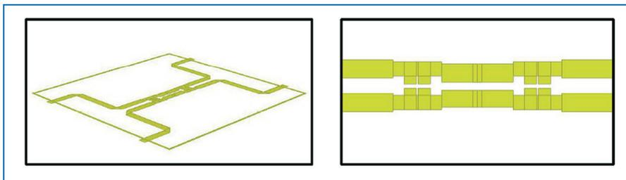
Figure 2: In order to further enhance the directivity, a multiple number of capacitors were placed on the coupler and their positioned optimized.
