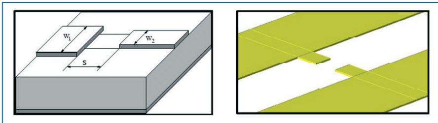
Figure 1: Symmetrical microstrip gap layout.
